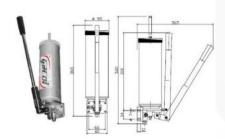
Hand pump used to feed progressive lubrication systems. Delivers oil with a viscosity greater than 50 cSt. and lubricants for 2 with a density by. NLGI.
